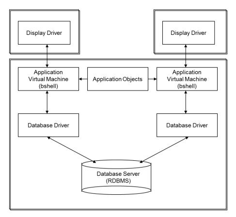
When two machines are available to be used as servers, two configurations are commonly used. In both configurations, the display drivers reside on the user workstations.
